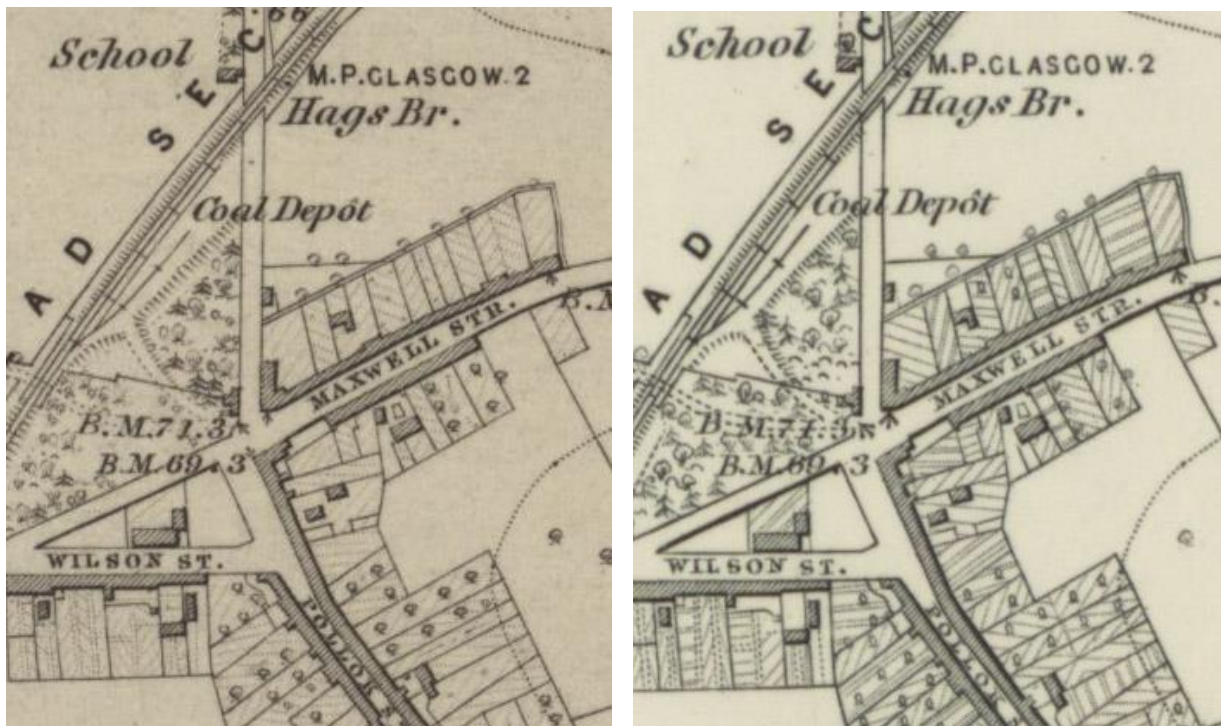
OS Six-inch to the mile, Renfrewshire, Sheet XIII, Surveyed 1858, Published 1863. These two sheets show how the garden ornament changed between states of the same sheet, reflecting different engravers, but with no change on the ground.
